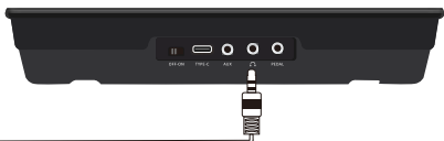
Schematic diagram of audio or headphones connection Audio output interface
